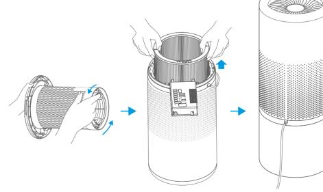
Rotate counter-clockwise to take out the wet curtain for replacement.
