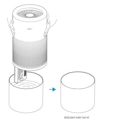
When removing the main unit for barrel cleaning and water route cleaning, please turn the power off to lift the main unit by hands and place it into a dedicated empty water barrel as shown above.
